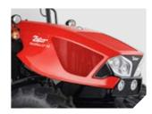
The new look is down to new plastics technology, which provides greater heat resistance and UV stability.
